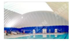
"best of both worlds" approach: the opaque fabric helps insulate the dome, reducing heating and cooling costs, while the translucent fabric provides pleasant natural light, reducing operating costs.
